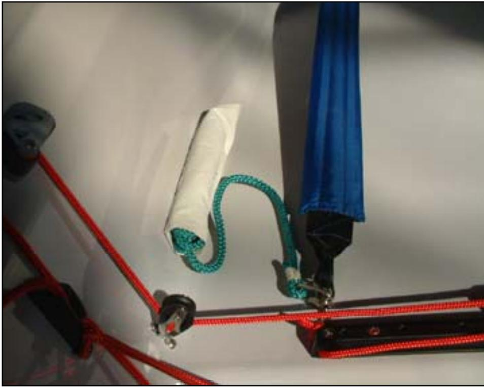
In light air, when you might be wanting to heel the boat over to the point where the gunwale could be in the water on the run, remove the pouch from under the gunwale and attach it to a second piece of Velcro hook on the sides of the tanks
