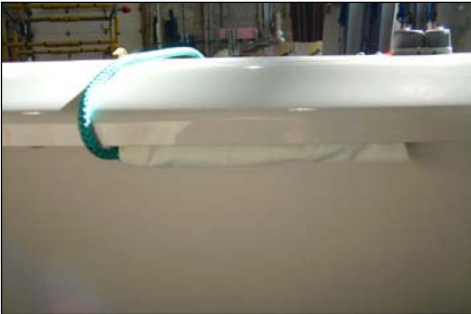
Once over the gunwale, it goes into the pouch which is attached by means of a strip of self adhesive Velcro "hook" permanently adhered to the underside the gunwale. The photo shows the pouch with the rope completely inserted.
