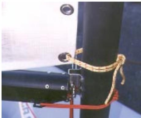
opposite side of the boom. This will prevent the boom crashing to the deck when you lower the sail! Tie the tack to the mast so that the sail is the same distance behind the mast as it is where it comes out of the track above. You should check this distance after pulling the outhaul tight.
