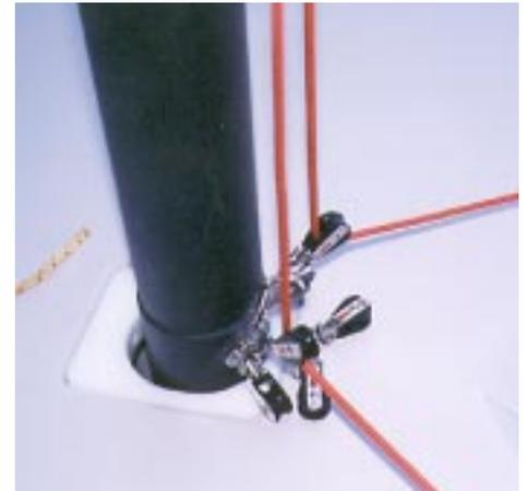
bottom of the halyard you will find a small bungee loop. Hook this around the small plastic standoff between
