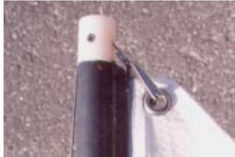
top, the angle at which the halyard pulls gets close to 45° which makes the last few inches of hoisting quite hard. Make sure you pull the halyard from about 3-4 ft. in front of the mast
