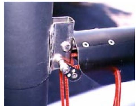
ends of the outhaul rope through the small blocks on the gooseneck and down to the TOP mini blocks which are attached on each side of the spar at the lower fitting. See below. From there, take them back to the TOP clamcleat on the deck and reattach the balls. Undo the temporary knot at the end of the boom and this completes the outhaul. Attached to the wire loop at the
