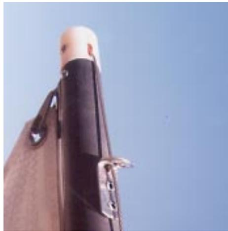
so that the ball goes through the opening in the lock without hitting the top of the fitting. Properly locked, it looks like the photo above.
