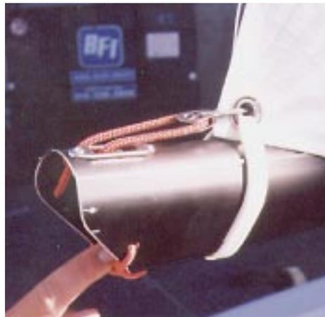
knot in the line to keep the sail out near the end of the boom. Slide the front end of the boom over the gooseneck pin as shown below then remove the balls and thread the two
