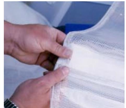
three battens insert through the slit in the batten pocket until they come up against an elastic at the front of the pocket. Force them further into the pocket then tuck the back end of the batten under the flap and release. The elastic will force the batten out against the leech.
